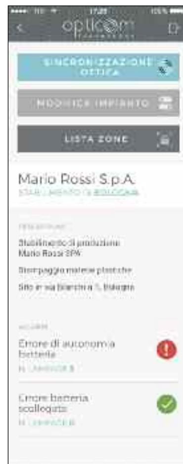
System details: Description of the system and of any lamp errors. The lamps can also be interrogated using the "optical synchronisation" push-button
